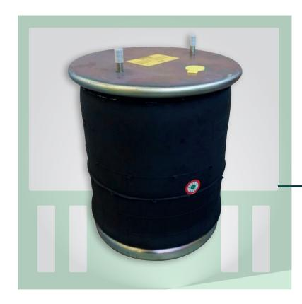
Air springs with shock absorbers constitute the air suspension of vehicles and trailers and they allow high performance in terms of comfort and safety. The air spring consists of a flexible casing made of rubber, containing compressed air inside and fixed to metal elements (or composite material).
