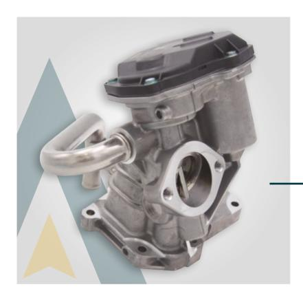
The **EGR valve** (Exhaust Gas Recirculation) is the main driver of the exhaust gas recirculation system. This system, by valve, ducts and radiators, is responsible for re-circulating a small part of the exhaust gases in order to reduce emissions.
