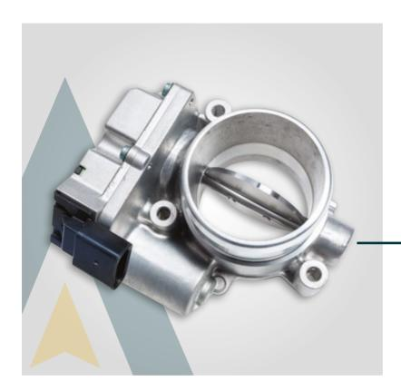
Mechanical and electrical throttle bodies regulate and optimize the engine idling speed. Along a main shaft, that is able to connect the inside of the heating unit with the external environment through the intake system, there is a throttle body, which regulates the flow of air inside the shaft.
