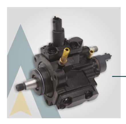
The Common Rail is a diesel injection system made of a single line, which connects the injection pump (a low-pressure pump with a high-pressure pump in series) to a series of electronically controlled injectors, with autonomy between management of injection pressure and time.
