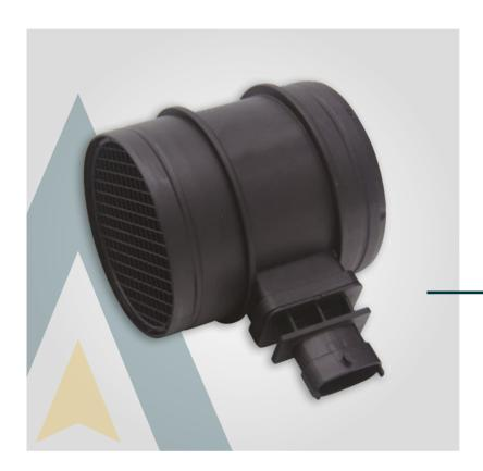
The air flow sensor is a flowmeter that measures intake air mass, speed and temperature, changing the air/fuel ratio. Thanks to this sensor it is possible to influence consumption and emissions.
